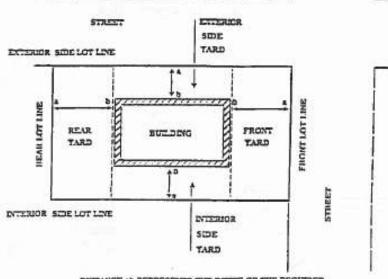
DISTANCE 45 REPRESENTS THE DEFTH OF THE REQUIRED TARD MEASURED AS LEAST BORDONTAL DIMENSION BETWEEN LOT LINE AND NEAREST PART OF MAIN BUILDING, DISTANCE 45 MUST BE THE MINIMUM DISTANCE SPECIFIED IN ST-LAW.
